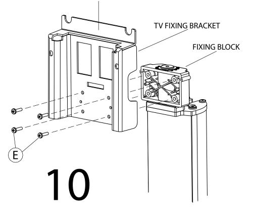
UNSCREW THESE PARTS FROM THE BACK OF THE TV. WITH ASSISTANCE ALIGN THE TV AGAINST THE TV FIXING BRACKET. REUSE THE PARTS TO SECURE THE TV TO THE BRACKET. DO NOT OVERTIGHTEN SCREWS.
